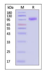
Human EGF R Protein, His Tag on SDS-PAGE under reducing (R) condition. The gel was stained with Coomassie Blue. The purity of the protein is greater than 95% (With <u>Star Ribbon Pre-stained Protein Marker</u>).
