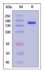
The gel was stained with Coomassie Blue. The purity of the protein is greater than 95% (With <u>Star Ribbon Pre-stained Protein Marker</u>).
