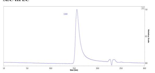
The purity of GMP GENPower<sup>TM</sup> NLS-Cas9 Nuclease (Cat. No. GMP-CA9S18) was greater than 95% as determined by SEC-HPLC.
